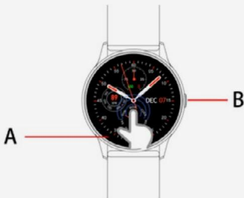
Your watch is controlled using both the full touch screen "A" and the pusher button "B", is the return key. Long press the pusher button for power on / off.
